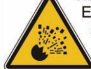
Explosive hazard. Do not pump gasoline, solvents, thinners or other flammable liquids. To do so can cause an explosion resulting in injury or death
